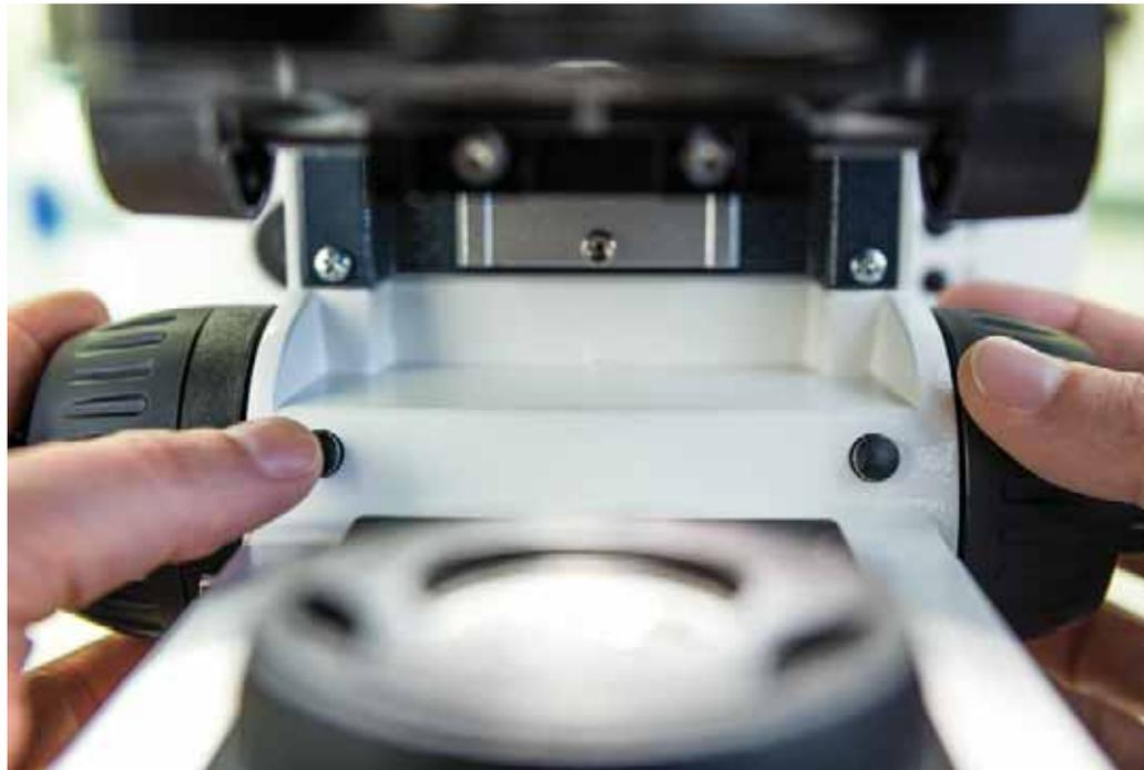
*Axioscope 5: Snap button for image acquisition on both sides
