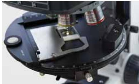
*Axioscope for polarization*
